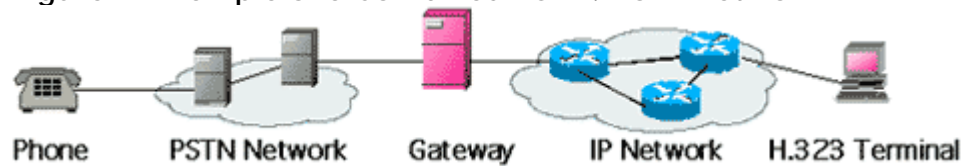
Figure 2. Example of a Combined PSTN/VoIP Network
