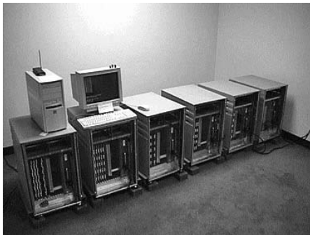
Fig. 3.17 Deep Crack — the hardware exhaustive key-search machine that broke DES in 1998 (reproduced with permission from Paul Kocher)
